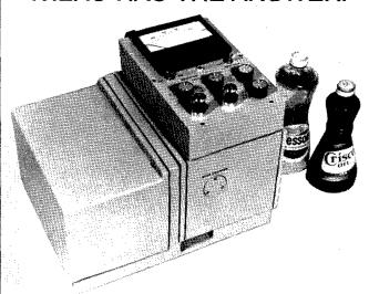
The Wilks On-Stream Hydrogenation Analyzer monitors the hydrogenation process used to convert edible oils to margarine and other food products.
